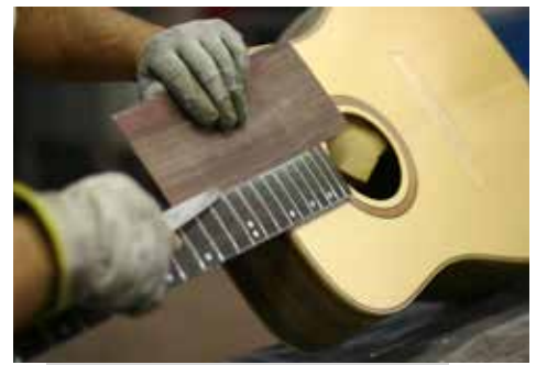
Process: frets installation
