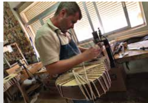
Process: assemblage and gluing of bindings
