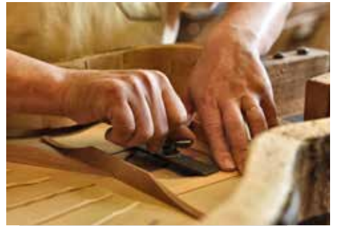
Process: adjustment of the bracing
